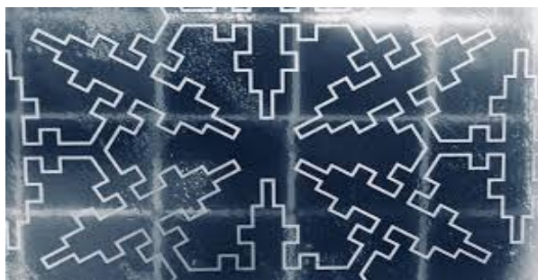
Fig. 4. The top view of the implemented antenna, which has dimensions of 20.4 cm×25.4 cm.
